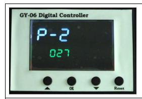
When SV and PV has a big difference, press  $\textcircled{\mathbb{R}}$  button for 5 seconds, and press  $\textcircled{\mathbb{R}}$  button again to adjust the temperature. If SV&PV has difference of 20 degrees, Press arrows " $\triangle$ " or " $\nabla$ " to set to 20.
