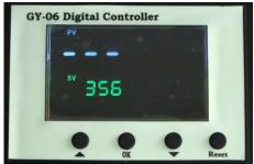
Press button, the temp light is on. Select with arrows the temperature according to different transfer material (Normally 180°C~200°C)
