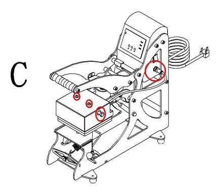
Fitted with locking screws, and insert the socket.
