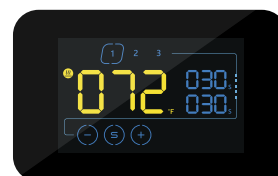
The controller is on. Three custom presets flash. Select one of custom preset to start your setting.
