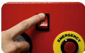
The Power ON/OFF Switch on the side of the press, turn the Power Switch ON.
